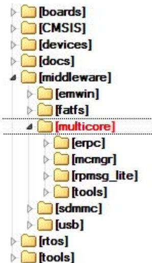
**Embedded Remote Procedure Call (eRPC)** The Embedded Remote Procedure Call (eRPC) is the RPC system created by NXP. The RPC is a mechanism used to invoke a software routine on a remote system via a simple local function call.
