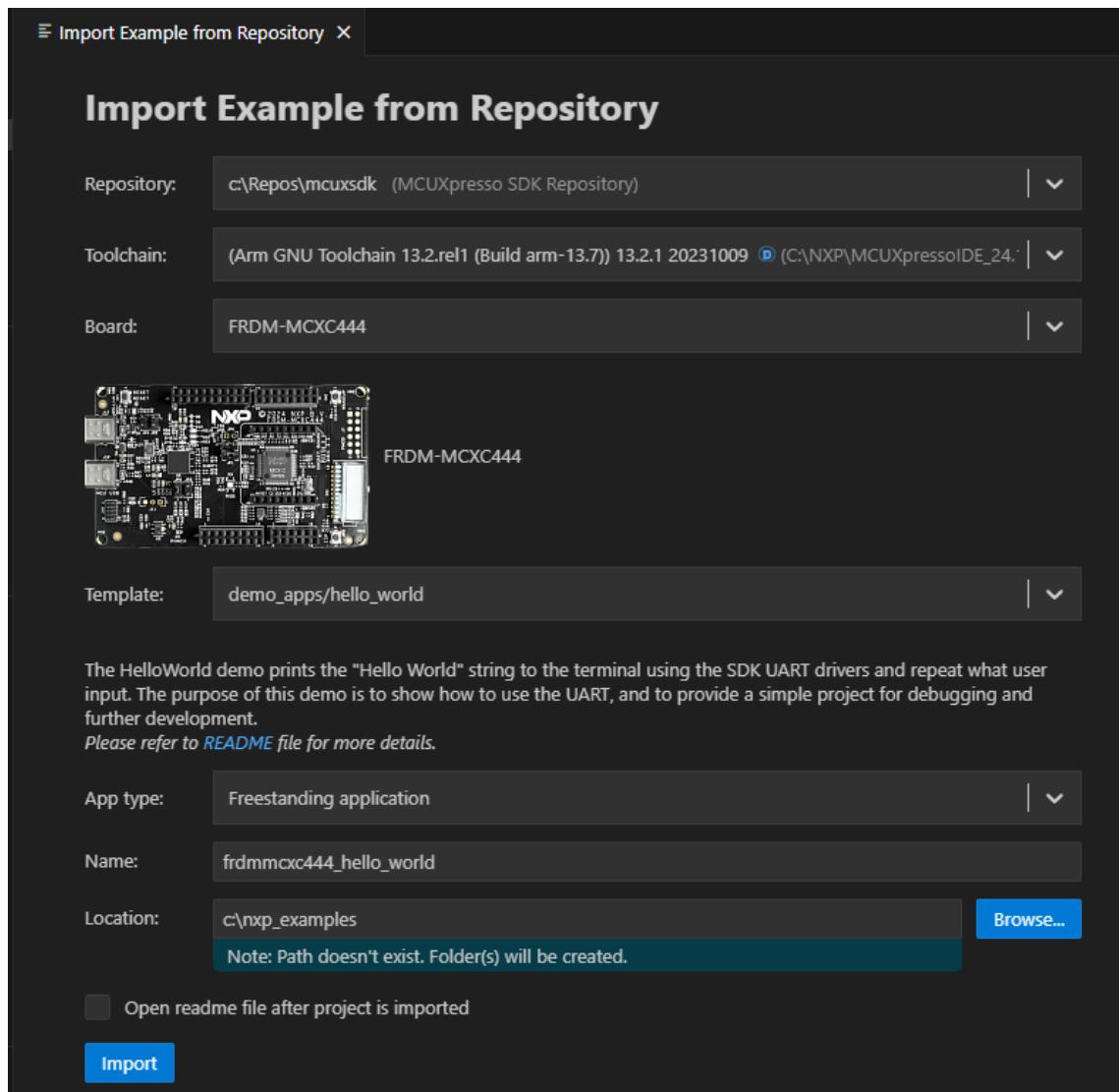
**Note:** The MCUXpresso SDK projects can be imported as **Repository applications** or **Free-standing applications**. The difference between the two is the import location. Projects imported as Repository examples will be located inside the MCUXpresso SDK, whereas Free-standing examples can be imported to a user-defined location. Select between these by designating your selection in the **App type** dropdown menu.
