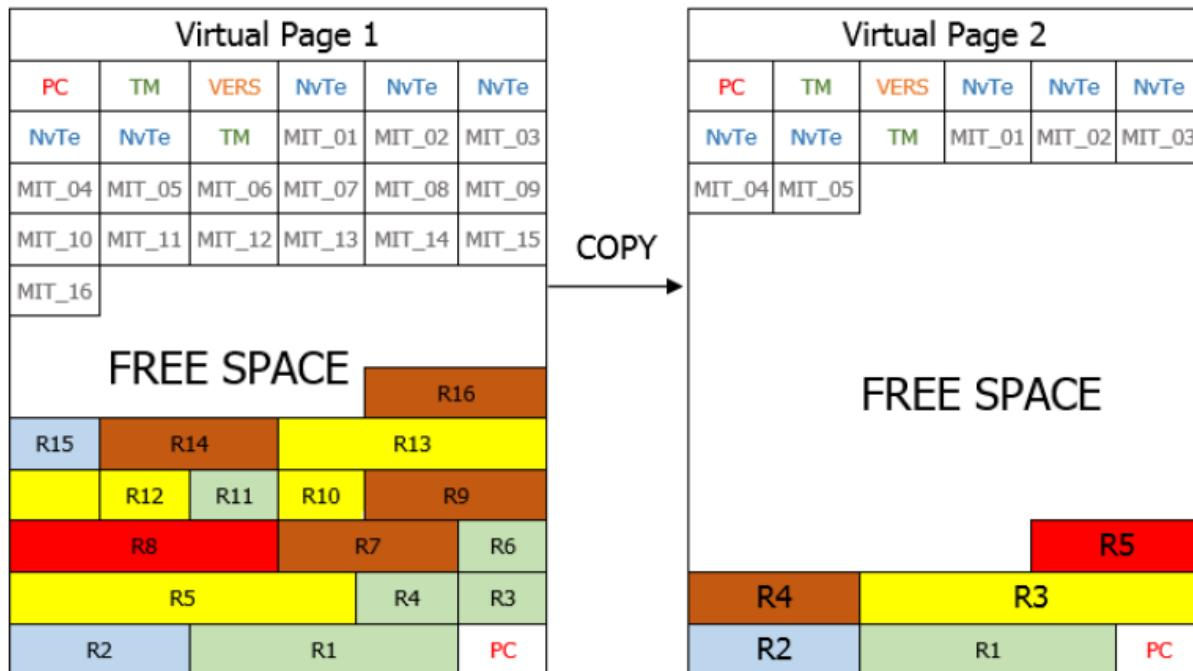
Finally, the virtual page 2 is validated by writing the PC value and a request to erase virtual page 1 is performed. The page is erased on an idle task, sector by sector where only one sector is erased at a time when idle task is executed.
