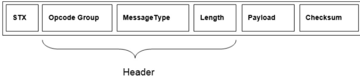
Below is an illustration of the FSCI packet structure when a virtual interface is used instead :
