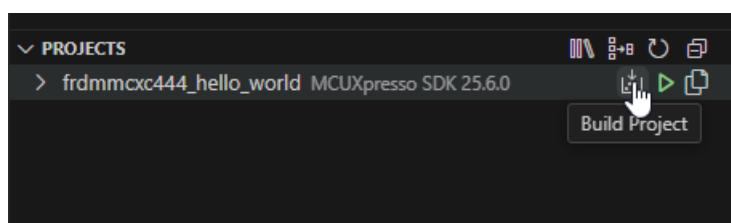
The integrated terminal will open at the bottom and will display the build output.
