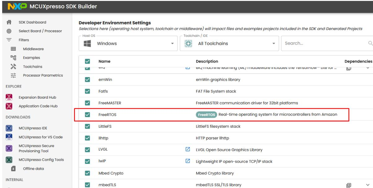
The FreeRTOS examples in MCUXpresso SDK zip packages are located in `<MCUXpressoSDK_install_dir>/boards/<board_name>/freertos_examples/` subfolders.
