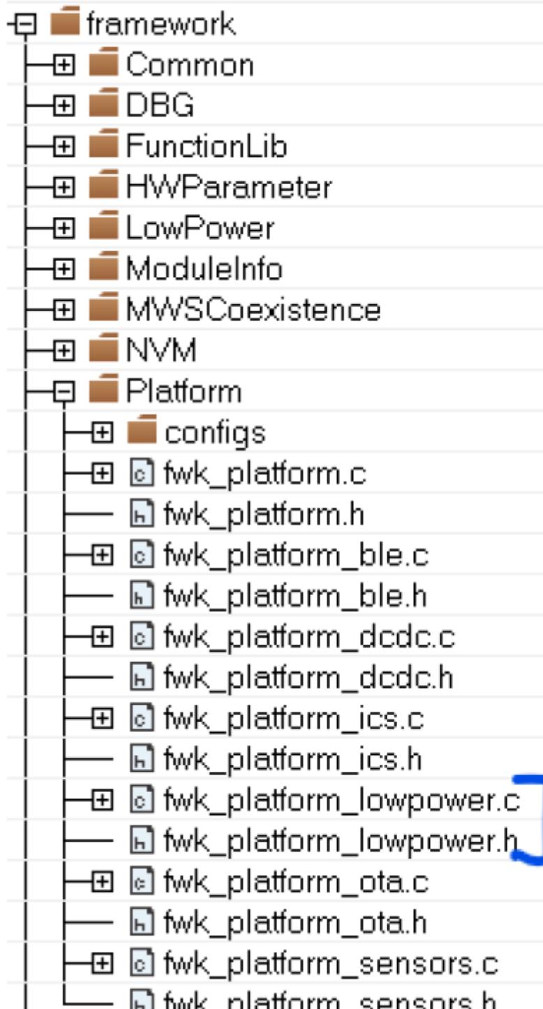
**2.1.4 - Low power board files** These files are located in the same folder that the other board files board.[ch]. Hence, it is not required to add any new include path at compiler command line.
