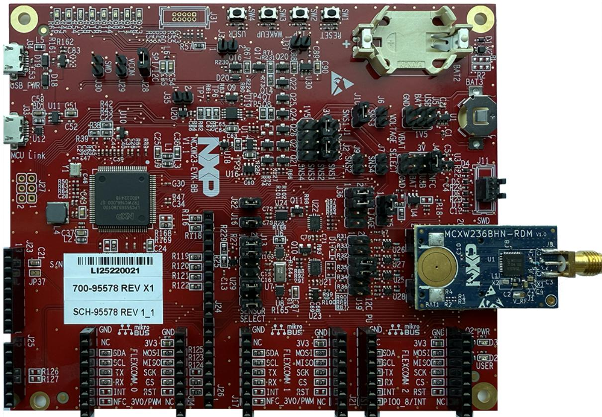
MCU device and part on board is shown below:
